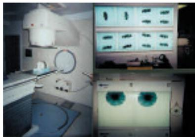
*An experiment of the new leaf sequencing software on the Elekta SL20 linear accelerator in the Department of Radiation Oncology at the University of Maryland School of Medicine (left). Film comparisons of delivered IMRT plans produced by the new leaf sequencing software and the commercial CORVUS 4.0 planning system (right).*
